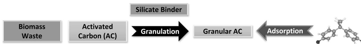
**Figure 1.** Process flow diagram of the preparation and use of adsorbent materials.
